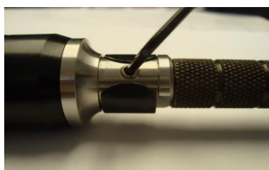
Fig 4 Lock the protective hose on the handpiece using a screw
